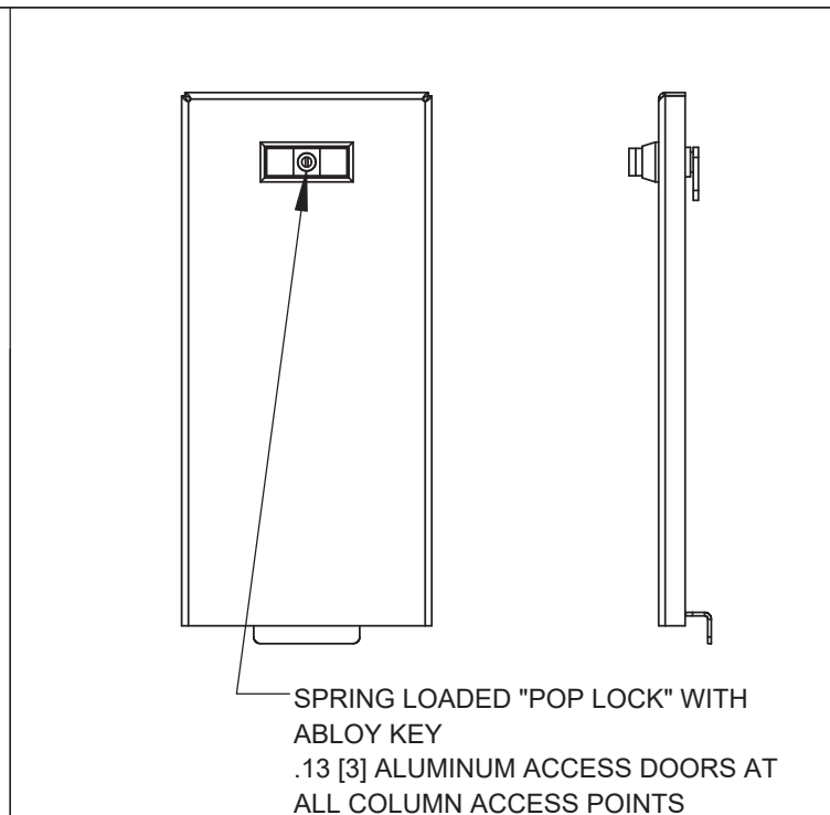
DETAIL E2 OPTIONAL HIGH SECURITY LOCK
